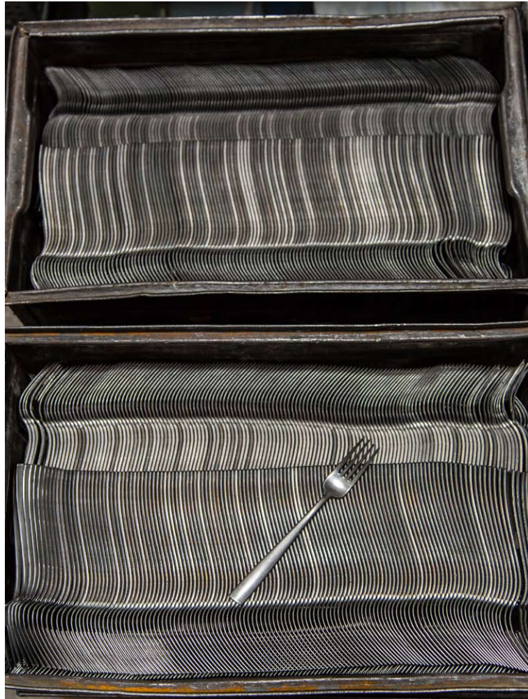
Particular phase to do just for the cutlery of 5 mm of thickness : heating in high level of temperture to make the steel softer during the phase of coniage
